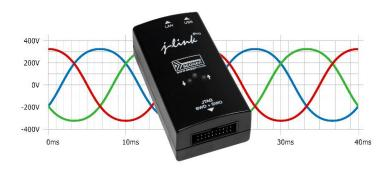
J-Scope is based on the newly introduced J-Link HSS (High Speed Sampling) feature, which makes it possible to continuously sample variables at extremely high speeds without affecting the real-time nature of the embedded device. Using the standard debug interface, it does not require any extra resources on the target such as memory, CPU time or extra pins.
