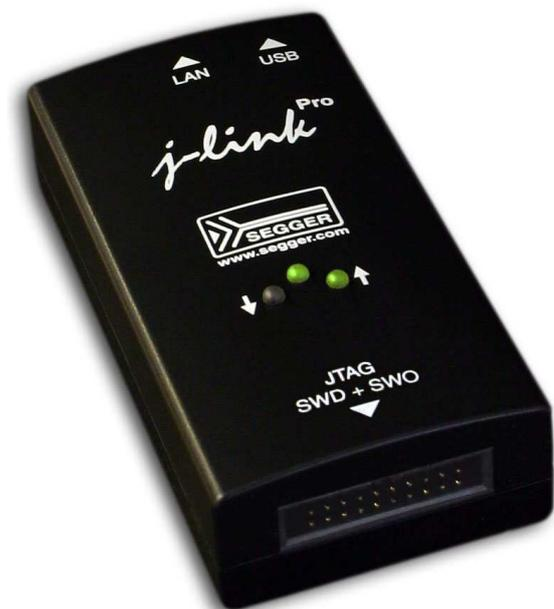
The SEGGER J-Link is the most popular debug probe on the market. It is tool chain independent and works with free GDB-based tool chains such as emIDE and Eclipse, as well as commercial IDEs from: ARM, Atmel, Atollic, Coocox, Cosmic, Freescale, IAR, Infineon, i-Systems, KEIL, Mentor Graphics, Python, Rowley, Renesas, Tasking and others. With the J-Link family, investments in the debug probe are preserved when changing compiler or even CPU architecture.
