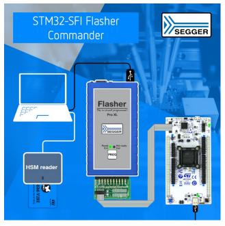
transfers the encrypted firmware image and the matching firmware decryption key (also in encrypted form) to the target MCUs to be programmed.
