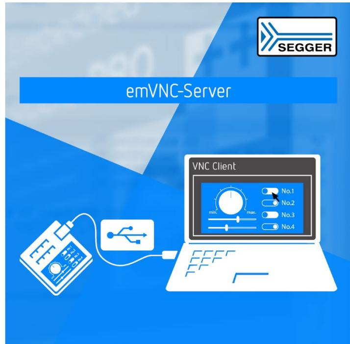
embedded systems with limited memory. emVNC-Server transports human input, such as mouse or touchscreen interaction, over USB to the embedded system, enabling control of the application, working in parallel with existing functionality.
