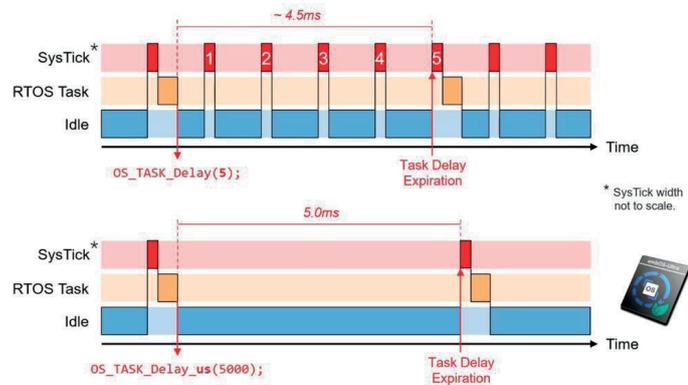
**Figure 2:** An example for the higher precision of embOS-Ultra. A delay of 5 ms can in reality only last 4.5 ms with a conventional RTOS, because a programmed delay cannot end between two system tick interrupts, but only with the next system tick interrupt, which then triggers
