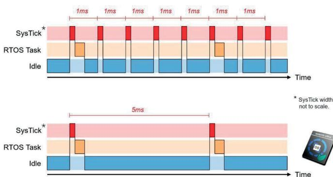
**Figure 1:** This graphic shows the difference between embOS-Ultra (bottom) and the conventional RTOS embOS (top): With embOS-Ultra, the CPU stays in energy-saving mode significantly longer and is woken up less often by interrupts (red). The result is more computing power for the application and less energy consumption. (Bild: Segger)
